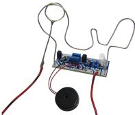
The matter is to pass a small wire loop through a thread wire with a lot of bends and obstacles. The person who touches the thread wire with the wire loop, will release an acoustic and optic signal. An interesting game for parties and for never-ending evenings.
