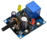
Adjustable time switch for switching operations from approx. 1 sec. to approx. 40 minutes. The device switches on after pressing the key and switches off again when the adjusted time has expired. The lapse of time may be interrupted any time with the reset key. Fitting case: G024 - Case With Fastening Straps approx. 72 x 50 x 41 mm
