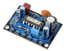
Small universal amplifier with a peak sound capacity of 2 W. A modern, low cost amplifier for many purposes. It works with an 8-pin DIP IC, the design is very small, so that this amplifier can be integrated into many devices. Fitting case: G027N - Plastic Case approx. 72 x 50 x 35 mm
