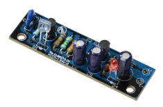
With the aid of this circuitry it is made possible to carry out functional tests of infrared remote controls used in TV-sets and video devices, etc. Whenever there is radiation of infrared beams on the Special-Sensor, the LED will light up and indicate that the infrared remote control is operated. As accessories is available our kit "B197 | Relay card 12 V/DC". This could be connected with the Infrared Detector and it is then possible to switch through the relay contact hade up to 3.0
