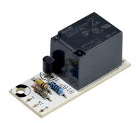
This relay card could be released with weak signals from approx. 5 mA upwards and will then switch a relay with a heavy current contact of 3 A. Ideal as switching amplifier for other kits, which have solely a light emitting diode as output and should switch other devices and machines through the relay contact. Fitting case: G027N - Plastic Case approx. 72 x 50 x 35 mm
