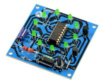
After releasing the push-button, the light signal rotates quickly at the 10 LEDs, slows down and then stops at random at one of the LEDs. During operation all LEDs shine except that LED that just receives the signal. That's why the luminous board looks very decorative. Fitting case: G100 - Display Case approx. 130 x 130 x 17 mm
