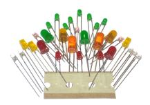
Lucky bag with different LED types This bag contains standard-LEDs of different colours and form. All LEDs run with a current of 10 mA or less. Each LED has to be set into operation by using a series resistor, which limits-according to the operating voltage- the current to 10 mA or less. The LEDs can only be used with direct voltage. The LEDs have different operating voltages, according to their colour.
