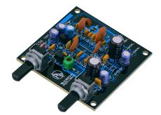
Kit for FM radio. The integrated audio amplifiers can drive an 8 ohm loudspeaker > 1 W. Pre-assembled SMD IC's and pre-printed coils simplify assembly. The kit can be powered by a 9 V battery.
