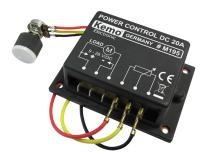
Power controller for controlling DC loads (DC motors, light bulbs, heaters, LEDs with current limiting resistors, etc.) The use of PWM (pulse width) control works well even with electric motors running at low RPM. Switching frequency: approx. 300 - 600 Hz (for motors, a humming noise may be heard). The control is via the supplied potentiometer or optional with an external control voltage 0 to 5 V/DC.
