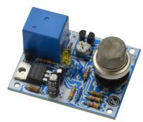
This instrument indicates gases such as alcohol, acetone, benzole, propane, carbon monoxide (contained in the smoke of fire). Perfect as alarm for gases and fire. Fitting case: G027N - Plastic Case approx. 72 x 50 x 35 mm
