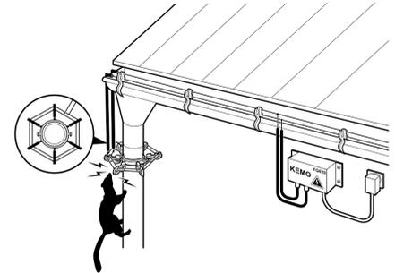
High voltage electric fence for mounting at gutters and downpipes against martens and raccoons in houses. The animals often climb up the downpipes and via gutters into the loft to nest there. An electric shock at this two pole electric fence should expel the animals effectively. A plug power supply 12 V/DC, output at least 100 mA or a 12 V car battery > 12 Ah is still required for operation (both is not included). In both cases the electric cable requires a barrel connector of 5,5 x 2,1 mm.
