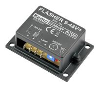
You may connect either incandescent lamps or LED lamps with operating voltages ranging from 9 to 48 V/ DC to the flasher. The flasher is then operated at the operating voltage of the connected lamps. The device is short-circuit proof. Adjustable flash period: approx.  $0.15 - 7 \, \text{sec}$ .
