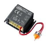
Regulates ohmic loads like heatings, etc. without additional need for interference suppression with pulses in zero crossing. Regulation takes place by switching on and off in pulses. It is, therefore, only suitable for heatings (heating plates, welding wires, thermal welding machines, ovens, etc.). Not suitable for motors and lamps (they would sputter and blink, respectively).
