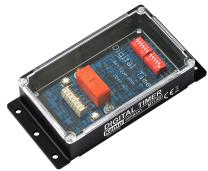
Timer with adjustable times between 1 second and 2047 seconds or 1 minute and 2047 minutes. The timer switches on after pressing the key and switches off again when the adjusted time has elapsed. The time lapse may be stopped at any time by using a second key. External push-buttons may be connected (not included). The timer can also be started by external control pulses (3 - 24 V / DC) or automatically after switching on with the connection of an Elko (22  $\mu$ F 50 V).
