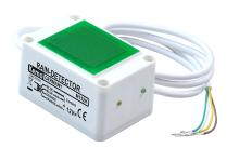
A relay connects if the completely insulated sensor plate gets wet (e.g. raindrops). In contrast to rain detectors with a metallic sensor, this sensor functions capacitively. That means it also switches when getting into contact with distilled water (completely clean rain). Skylights may then be closed with it, canvas blinds may be pulled in or rain is just indicated. 2 installed LEDs indicate the function. The sensitivity is adjustable.
