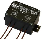
This solar charging controller is connected between a solar cell 12 V/DC (open circuit voltage 14 - 30 V/DC) and a battery 12 V/DC to prevent an overcharge of the battery. LED displays for "battery full" (approx. 14.4 V/ DC) and "charging".
