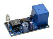
The kit switches on/off a relay at light and darkness (shadow). Usage: Whenever the light beam of a lamp on doors, windows, etc. is interrupted by a person, the relay connects. Also suitable as twilight switch. Fitting case: G027N - Plastic Case approx. 72 x 50 x 35 mm
