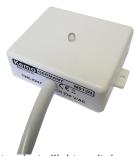
This electronic twilight switch connects automatically by means of an installed relay lamps (e.g. energy saving lamps) or other consumers at nightfall and off again at daybreak. The module may also work the other way round: on at daybreak (for advertising displays, fountains etc.) and off at nightfall. Floating loads up to 3 A may be switched.
