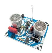
An LED lights up if a body approaches the ultrasonic sensors at a distance of 10 - 80 cm (depending on the size of the body). Use: parking-in assistance for cars in garages, alarm signal for persons or animals staying in a certain area. Operating voltage: 9 - 12 V/DC. The device works according to the same principle as the ultrasonic echo ranging of bats!
