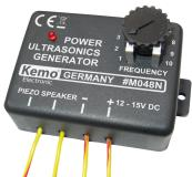
Through ultrasonic sounds it is possible to scare away animals and insects: e.g. rats, mice, martens, wild rabbits, mosquitoes. If mounted at the car, roe will be put to rout (decreased danger of accidents). For connection of a piezo-treble loudspeaker. The module is an ideal aid to scare away destructive animals out of your pantry, kitchen, storehouses, garden, etc. Also to be used as dog whistle. There are some birds species which will be scared away out of your fruit trees.
