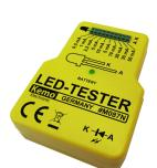
With the aid of this test module it is made possible to carry out tests of wired light emitting diodes in order to check function, brightness, colour and polarity. In order to facilitate selection of LED's of equal brightness, there have been placed two test sockets with the same currents (5 mA/10 mA) side by side. Necessary: battery 9 V (alkali).
