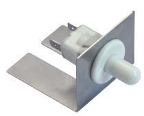
Please place the switch in a way, that the pin is 60 - 80% pressed when the hood is closed. Then the connected anti marten device turns on. The pin must not be pressed to the limit, because the switch can then be broken when the hood is slammed vigorously (the pin then strikes against the stopper and pushes the switch bottom out).
